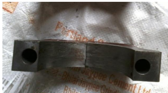
Fig. 3 Cracked MB-Cap Model.
